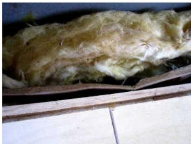
Install horizontal furring strips along the walls with a full inch Polyiso in between, with the reflective barrier facing the skin of the van. The additional 1 inch air space between the foam and the outside skin prevents heat transfer through conduction. The small air gap also limits the possibility of convection and the reflective barrier eliminates most of the radiated heat. You can add another 2
