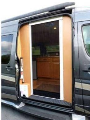
A new trend in Class B RV's is the installation of a permanent screen door inside the sliding side door. At your campsite, the somewhat awkward side door could
