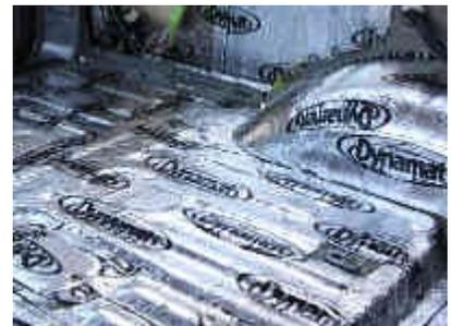
Just 25% coverage will limit the redistribution of sound through vibration, but not necessarily the transmission of noise. Butyl and rubberized asphalt are chemical compounds and their use in a confined space may have environmental consequences. These are heavy materials and will easily add 100 lbs to the overall weight of the vehicle.
