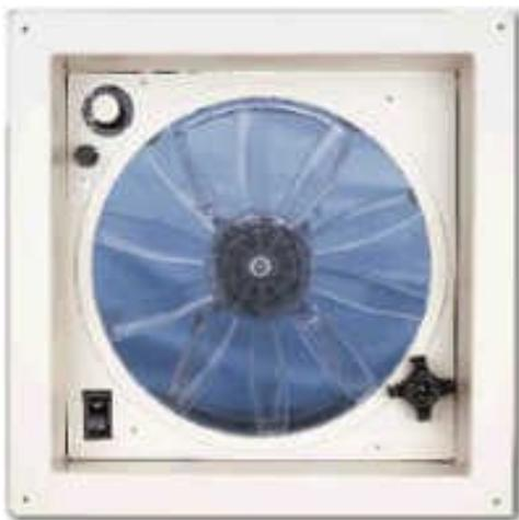
The roof vent plays a pivotal role in ventilation, yet at the same time is a major source of heat loss. It is exposed to the sun for most of the day, especially when the van is equipped with solar panels.
