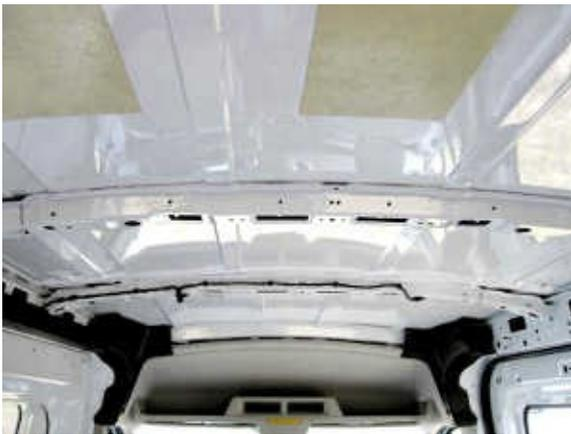
Some of the new European cargo vans are already equipped with some basic 'noise reduction padding', but adding some insulation at specific locations around the van may improve the acoustic qualities of the van considerably. Despite the implied need, acoustic insulation for RV's may be overrated, as these vehicles tend to be stationary and not driven on a daily
